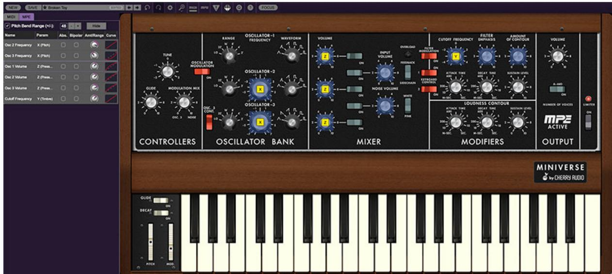
Miniverse supports MPE, short for "MIDI Polyphonic Expression." It's a specialized MIDI protocol enabling multidimensional controllers for controlling multiple parameters of individual notes. MPE specifies the MIDI messages used for three dimensions of control, regardless of how a particular controller physically expresses them. MIDI channel 1 is used as a master channel for global pitch bend, aftertouch, etc.; MPE utilizes MIDI channels 2-15 for the remaining controller data.
